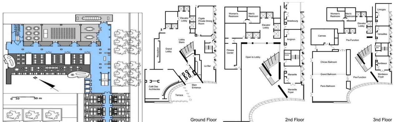
Fig. 6 Spatial layouts of conference centers – on the left: single-floor system in Andel's Hotel in Czech Republic, on the right (3 drawings): multi-floor system in "Sofitel Chicago Water Tower", USA (drawings based on (Vickers 2005, p. 34), (Water [...], 2013))
