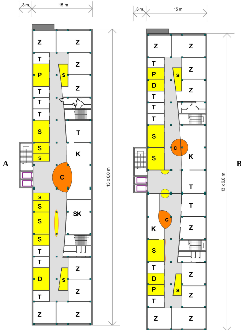
Figure 5. Adaptation to the nodal concept: A – higher floors – first variant; B – higher floors – second variant. C – ‘attractor centre’, I – individual booths, Z – team spaces, S – meeting spaces, T – touchdown, K – retreat / café, D – printing and copying services, P – storage, SK – conference room.
