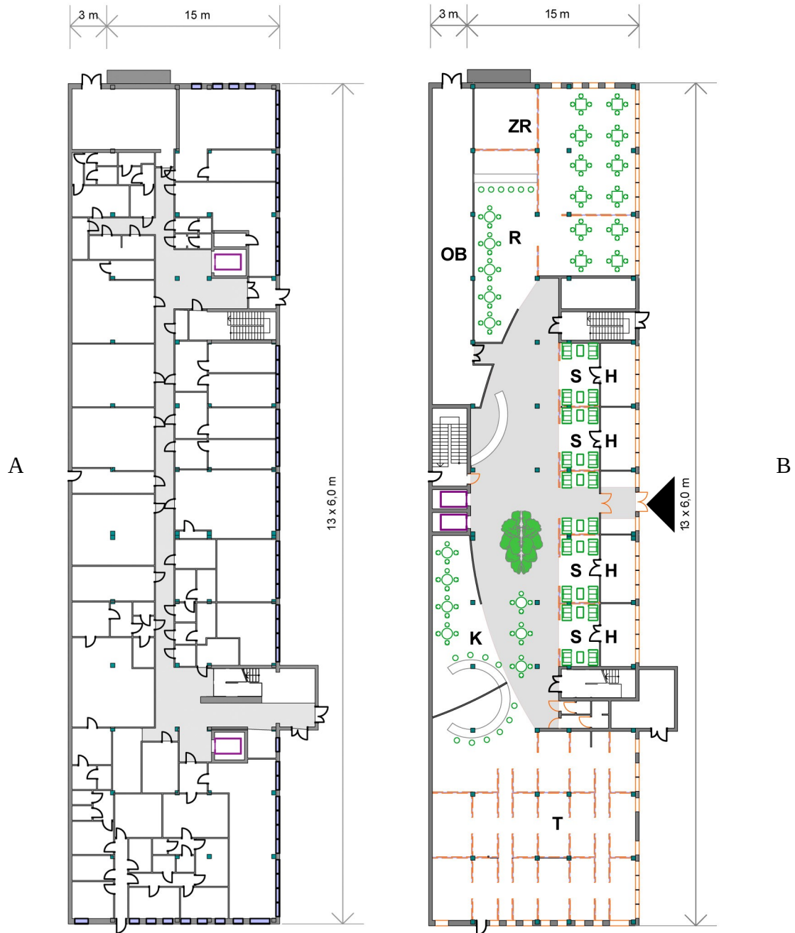
Figure 6. Adaptation to the nomadic concept. A – ground floor – present state; B – ground floor – adaptation. T – touchdown, S – meeting spaces, K – café, H – retail / services, R – restaurant, SK – conference room, OB –service spaces/ plant rooms, ZR –ancillary areas/ kitchen.
