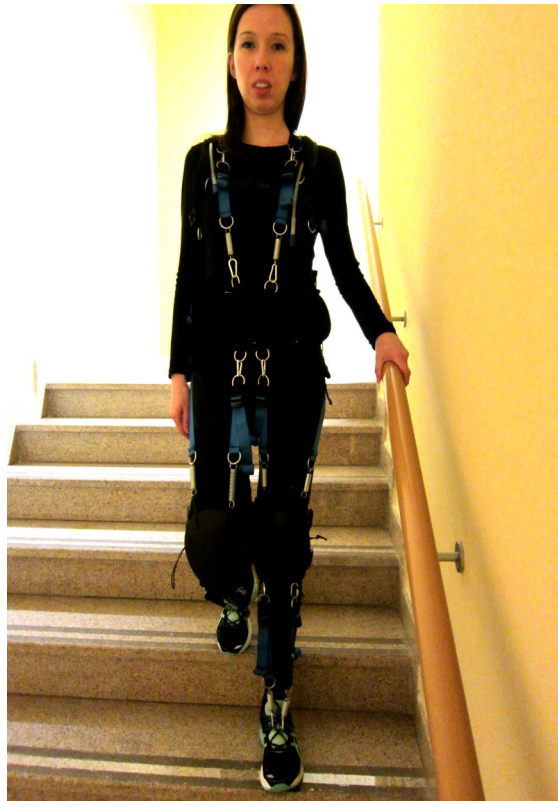
Figure 8. View on the walking system prototype. High springs elongation is visible, at the top straps of the right leg. It is visible that the muscles works is supported by the system. (Tester and demonstrator: K. Moshalov)
