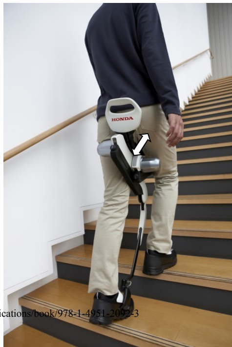
Figure 3. "Walk Assist" system, build by Honda. The system helps to rotate the legs around the hip joint. System is attached to the user body by the "belly" belt and tight straps. The belt must be quite stable to transfer the horizontal reactions. (The photo was adapted from:
