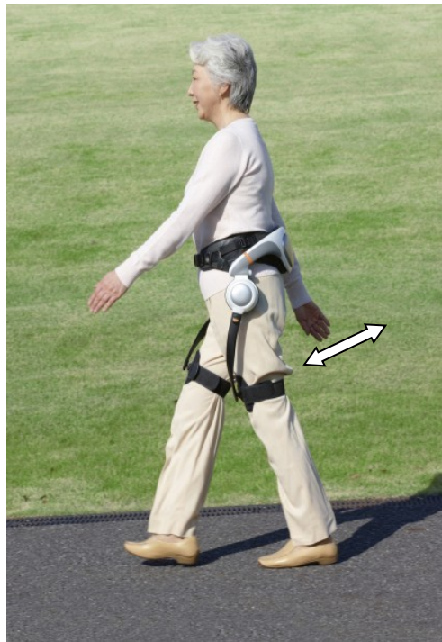
Figure 3. "Walk Assist" system, build by Honda. The system helps to rotate the legs around the hip joint. System is attached to the user body by the "belly" belt and tight straps. The belt must be quite stable to transfer the horizontal reactions. (The photo was adapted from:
