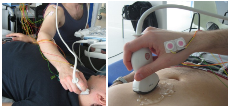
Figure 11. Example of in vivo test: A) Vascular application CCA; B) Abdominal application AA scanning
