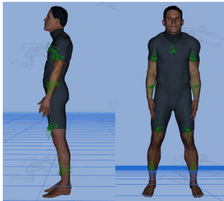
Figure 3. The Santos Avatar in Neutral Position. The forces (Lift and Drag) are represented with green line.
