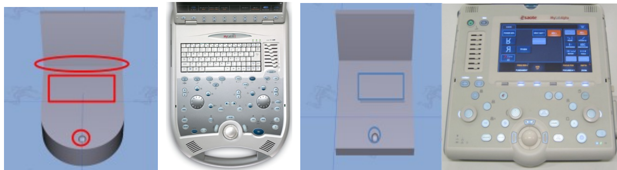
Figure 3: Left: MyLab30CV Console, presented as a simplified .obj model imported in the Santos Environment, and a picture of the real interface. In red are shown the different areas of investigations for the simulation conditions of the Left Hand. Right: MyLabAlpha Console presented as a simplified .obj model imported in the Santos Environment, and a picture of the real interface. In this case, the investigated zones for the simulations are shown in blue.
