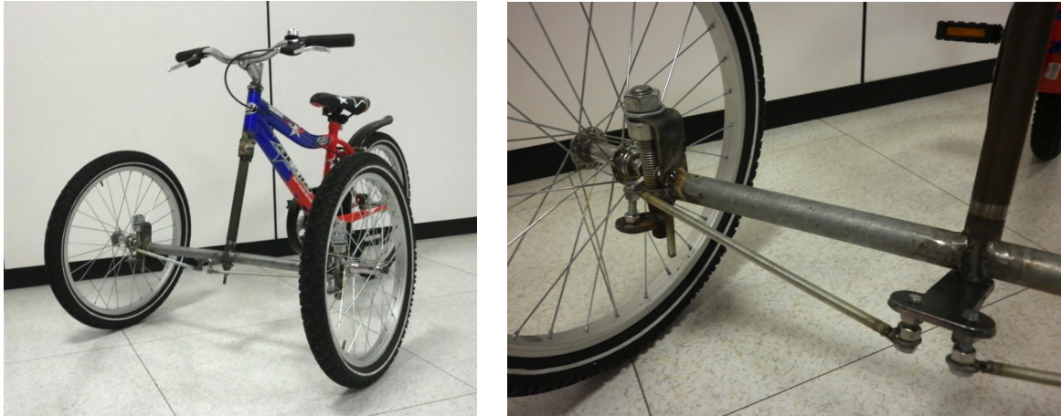
Figure 3. First functional prototype developed, front view and detail of the steering mechanism.
