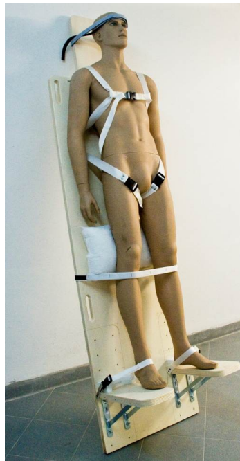
Figure 3. Wook mock-up and harness system
