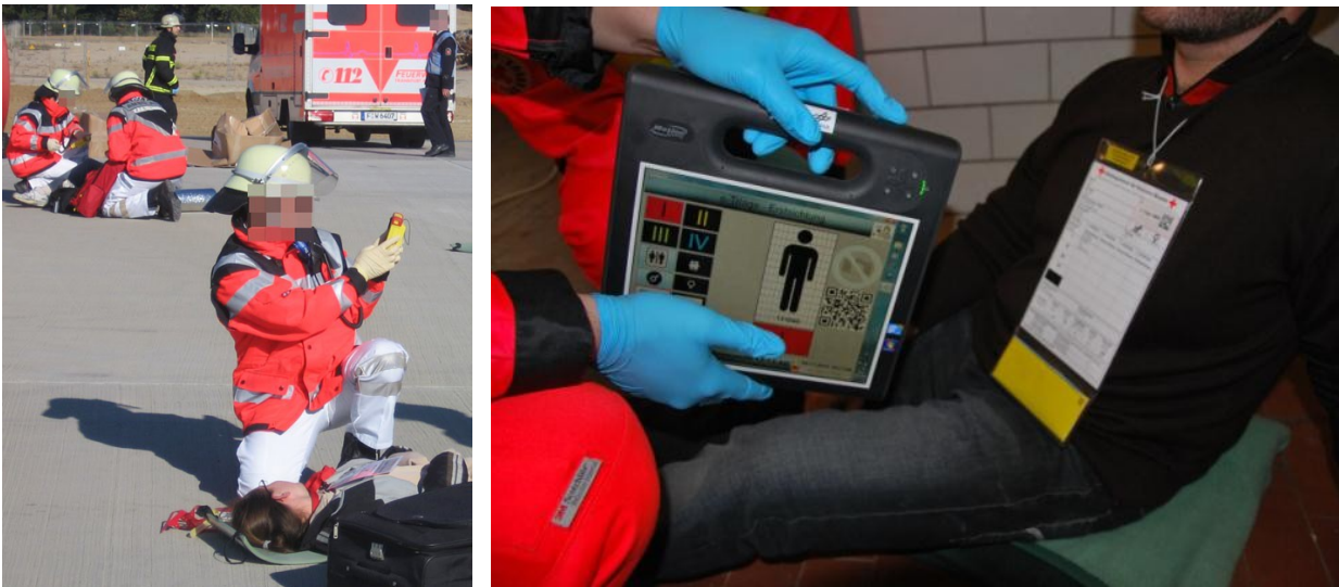
Figure 2: (left) Documenting triage results with a PDA (Ellebrecht & Latasch, 2012) and (right) scanning a triage tag with a tablet PC (Chaves et al., 2011)
