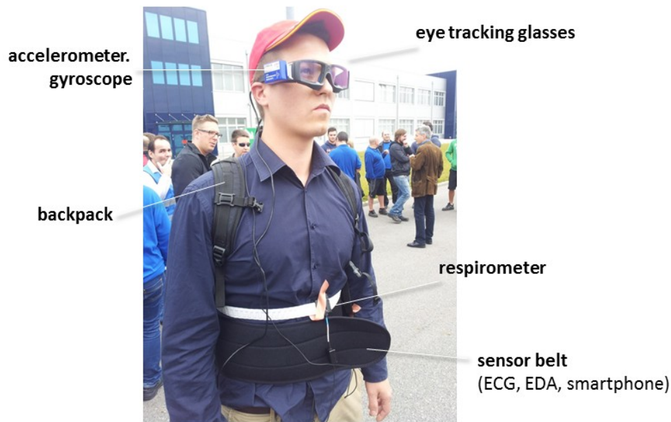
Figure 1. Participant of the user study with wearable sensor interface for human factors analysis.
