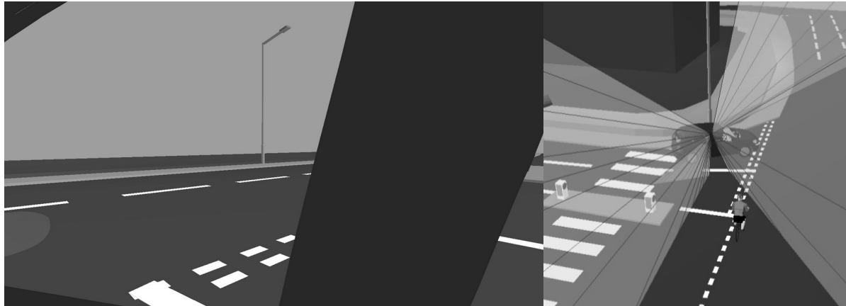
Figure 10. The view of the driver (99 th %ile Dutch male) of the Volkswagen Touran in the direction of the cyclist (direct vision on the left, volume projection on the right).
