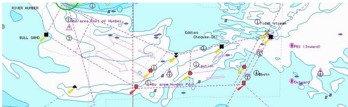
Figure 1. The TTS outside the river Humber in the U.K. Very deep draught ships has to transit the northern part of the inbound lane going both in and out due to limited under keel clearance. In such cases where an outbound ship uses the inbound lane, inbound ships are instructed to use “the southern part of the inbound lane”. This instruction is often misinterpreted to “use the southern (outbound) lane”
