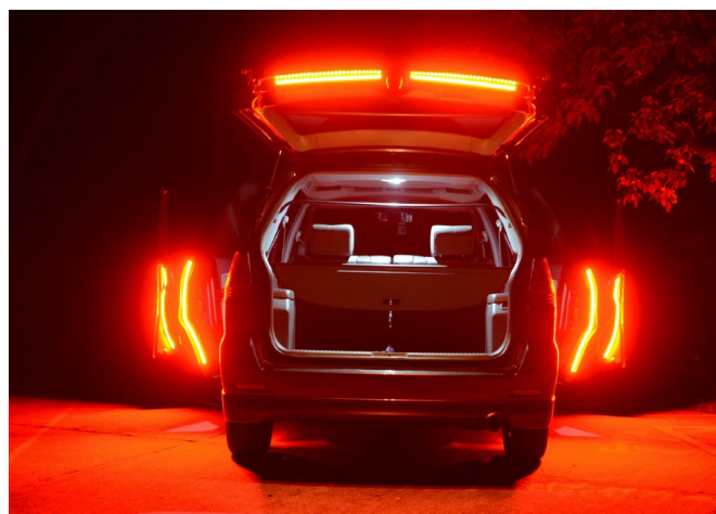
Figure 9. Alert from LED lights after car doors are opened.
