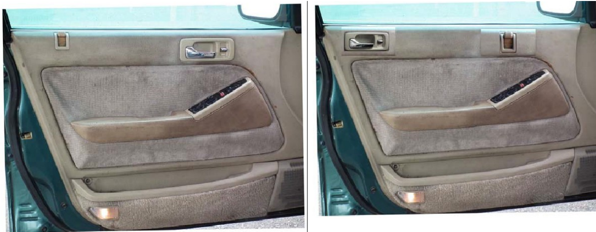
Figure 8. Change in the position of car door locks.
