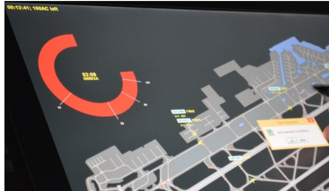
Figure 6. The clock on the ground surveillance display feeds back the head start to the operator.
