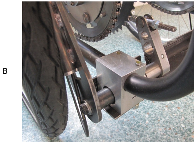
Figure 3. Moveable mounting of the levers axis of rotation: lever (1); wheelchair frame (2); levers axis rotation fastening moveable along the wheelchair frame (3); back wheel (B); levers axis of rotation (4).
