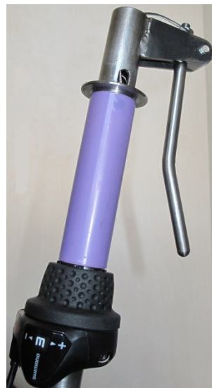
Figure 4. Grip with manipulation devices: service brake handle (5); grip with ride direction change (6); Shimano gear shifter (7).
