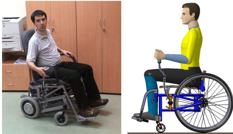
Fig. 1 Prototypical construction of an electric wheelchair and a wheelchair driven by levers
