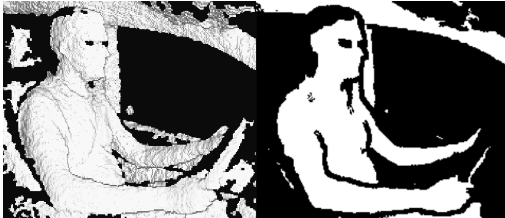
Figure 1. Left: visualization of a depth frame. Right: The corresponding mask with enhanced boundaries between objects, computed using our framework
