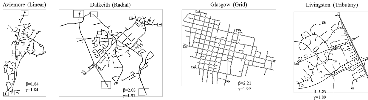
Figure 2. Traffic microsimulation models of Aviemore (tributary), Dalkeith (radial), Glasgow (grid) and Livingston (tributary).
