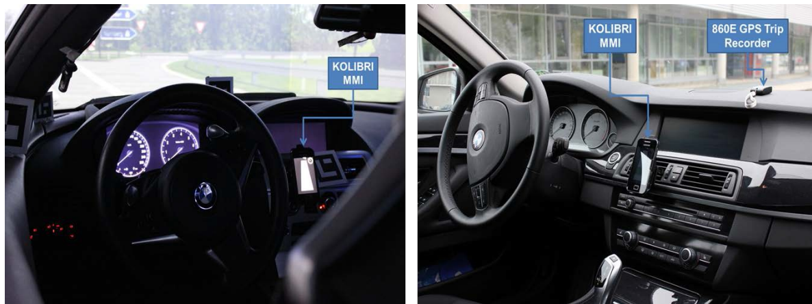
Figure 6 Mounting of the smart phone in the simulator (left) and the vehicle for the field test (right)
