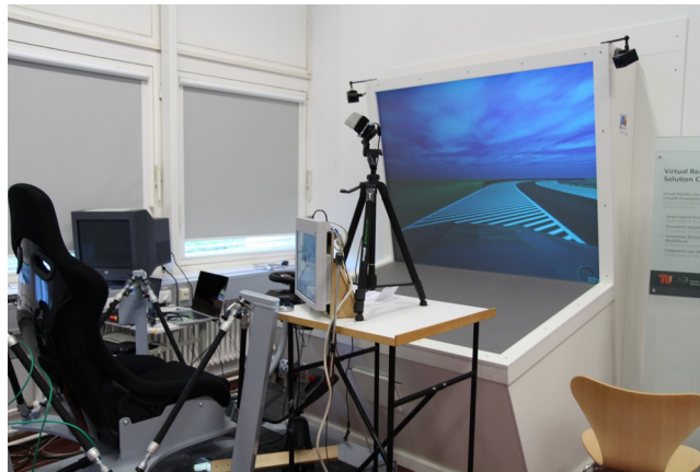
Figure. 1. Driving simulator and holobench at the VRSC
