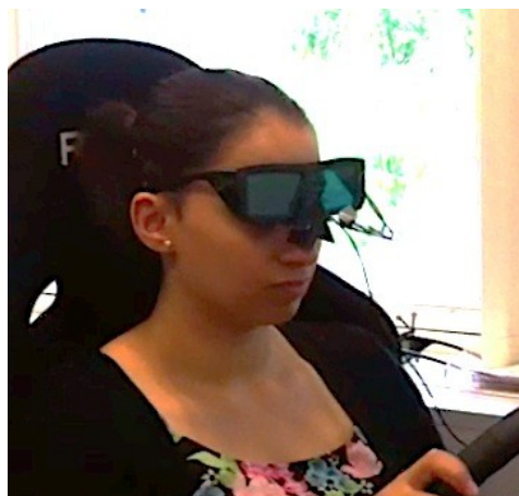
Figure 2. Self-built combination of eye-tracking system and shutter glasses
