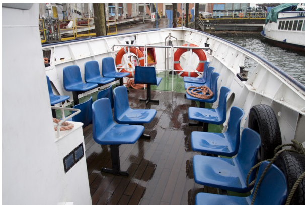
Figures 12 and 13. Open passenger areas on the prow (left) and on the stern (right). On the right picture, the door coaming is clearly visible. The pictures were shot during maintenance operations in the shipyard.
