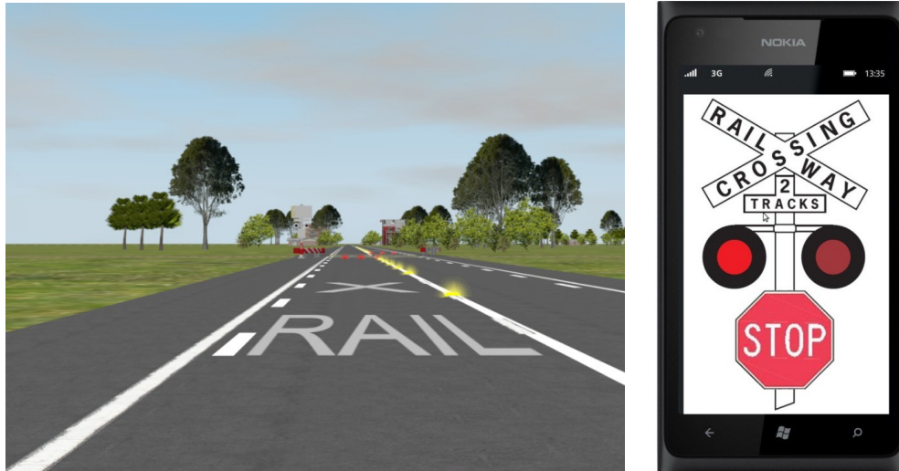
Figure 2. On-road intervention and visual in-vehicle ADAS.
