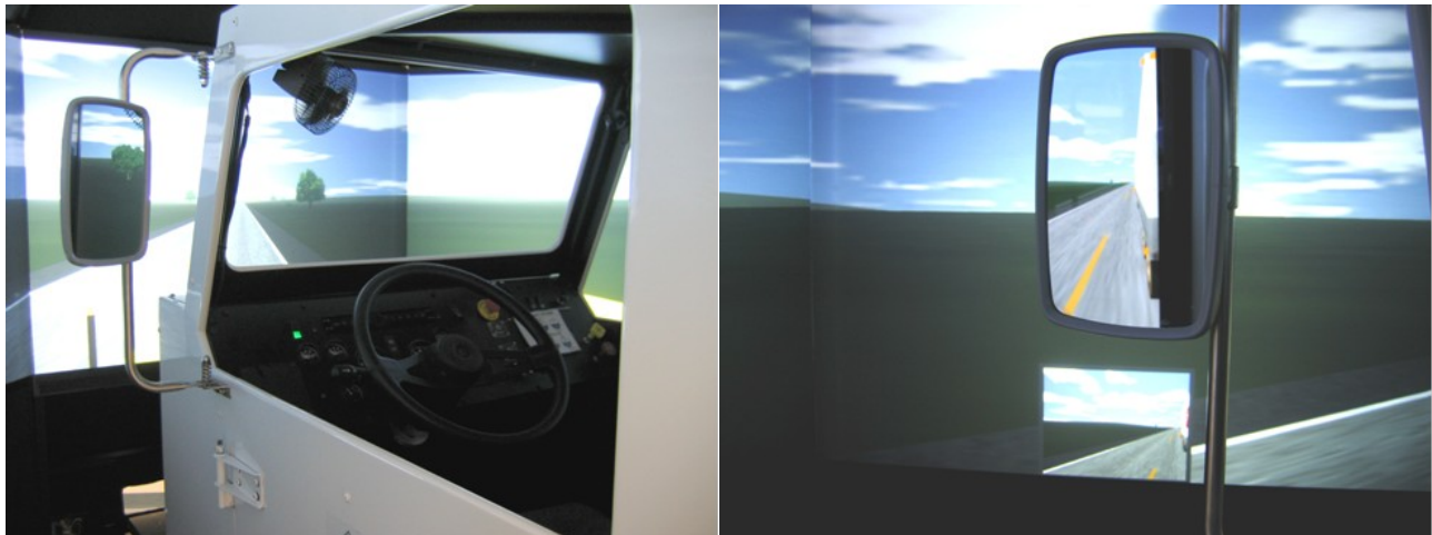
Figure 1. The TT-2000-V7 driving simulator (left) and the rear visual channel as viewed through the simulator mirrors (right).
