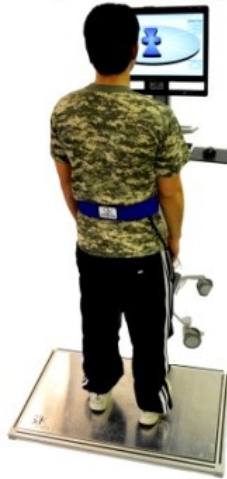
Figure 3. Patient standing on force plate using tactile feedback to improve balance performance.
