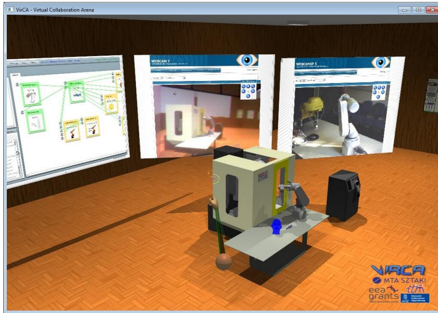
Figure 1. A simple virtual room in VirCA. The real world robot can be seen in the rightmost browser window, while its virtual model is in the middle. In the browser to the left, the modular structure of VirCA can be seen. Each box is a specific module that can be connected to others thus creating very complex systems.
