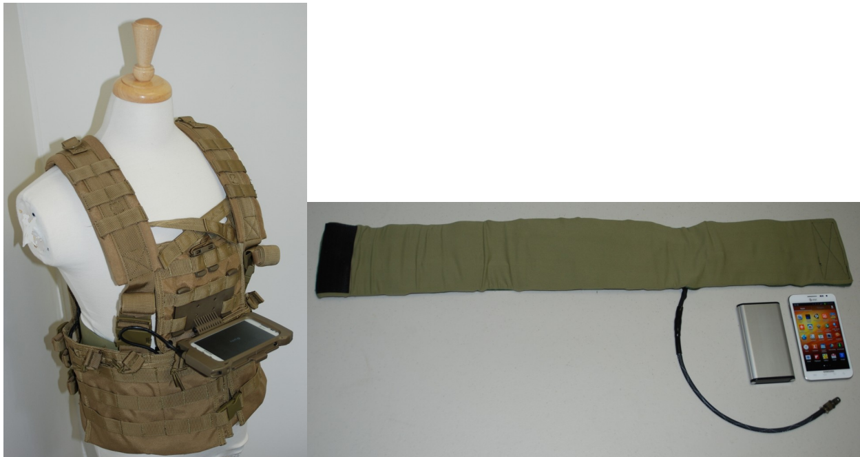
Figure 9. EAI prototype NavCom dual-row tactor belt, battery controller, and GPS sensor
