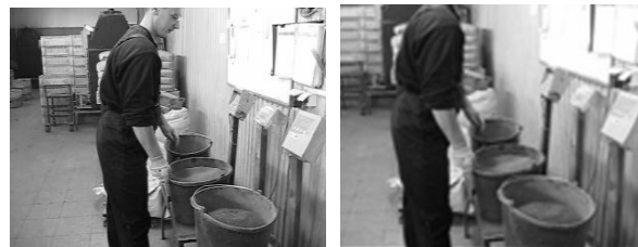
Figure 4: Weighing and transporting resin into mixer - 38kg per bucket
