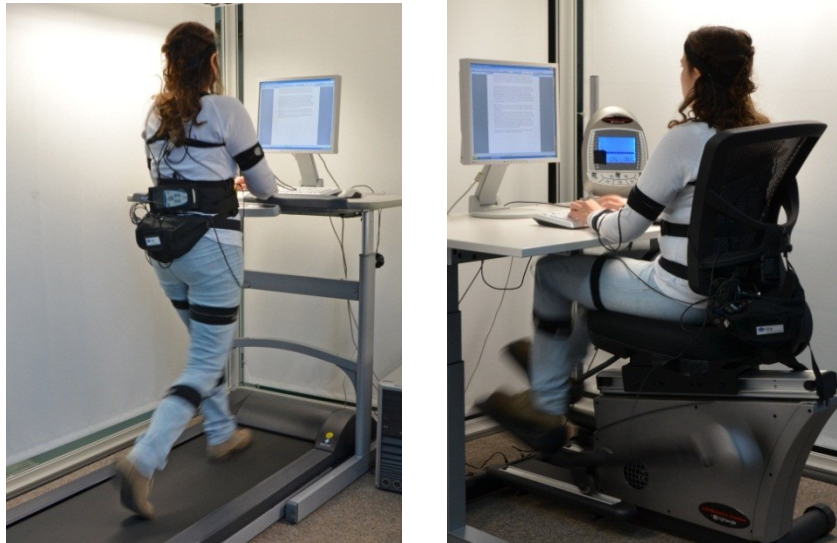
Figure 1. The Treadmill Desk (left) and the LifeBalance Station (right) in the laboratory set-up with a participant wearing the data capturing equipment
