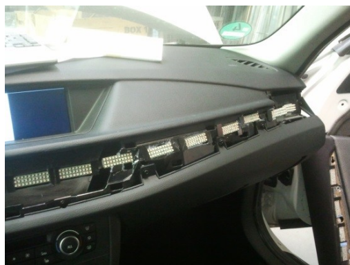
Figure 2a. Adaptive interior lighting mounted in the dashboard (left picture), red lighting of dashboard and door trims adapted to red shirt of driver detected by camera.
