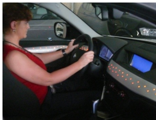
Figure 2a. Adaptive interior lighting mounted in the dashboard (left picture), red lighting of dashboard and door trims adapted to red shirt of driver detected by camera.
