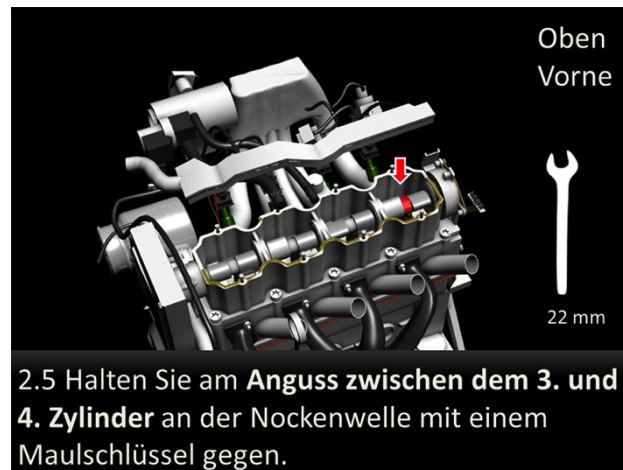
Figure 2. A working instruction the 3D model of the manufacturing object, textual instructions, graphical representation to the tools and a textual position indicator.
