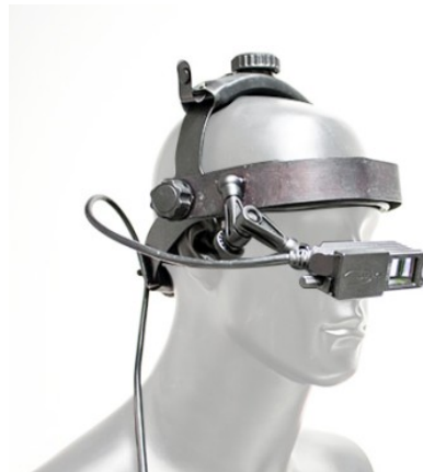
Figure 1. Working instructions were displayed on a monocular HMD Lite-Eye LE A750.
