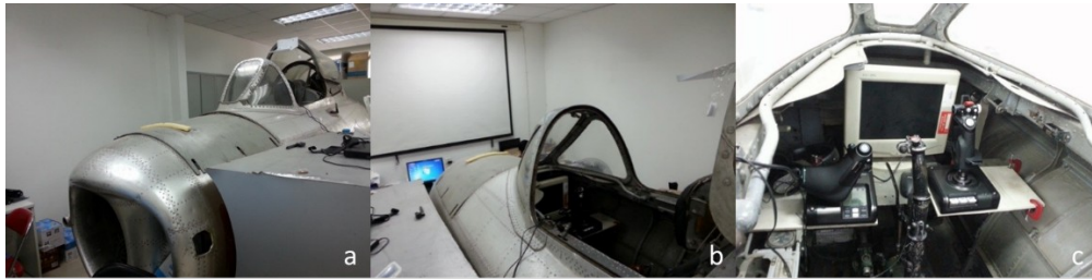
Figure.1. a shows the front view of the cabin; b shows the side view of the cabin; c shows the layout of the joysticks in the cabin.
