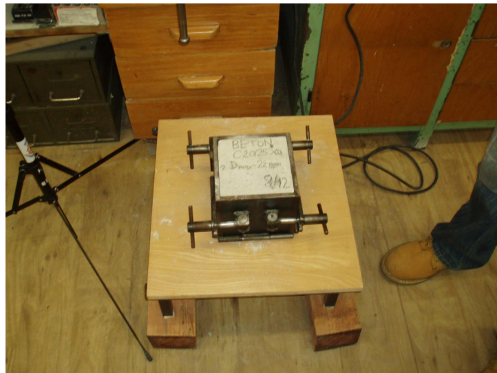
Figure 1. Sample fixation for vertical drilling (Hrazdilek and Fiserova, 2012)
