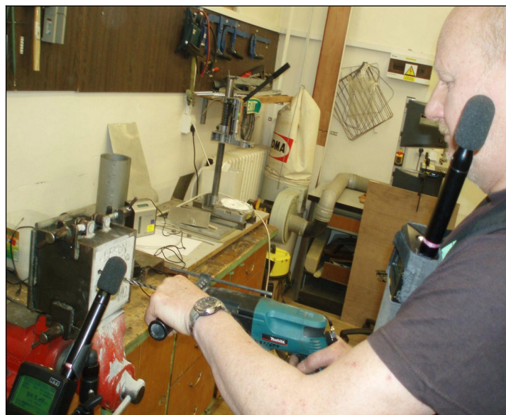
Figure 2. Sample fixation for horizontal drilling (Hrazdilek and Fiserova, 2012)
