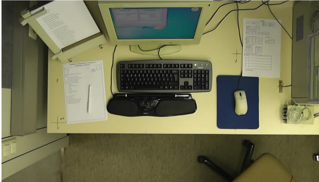
Figure 2. Rollerbar mouse with wrist support in front of a standard keyboard and optical wheel mouse on a mouse pad next to the keyboard.
