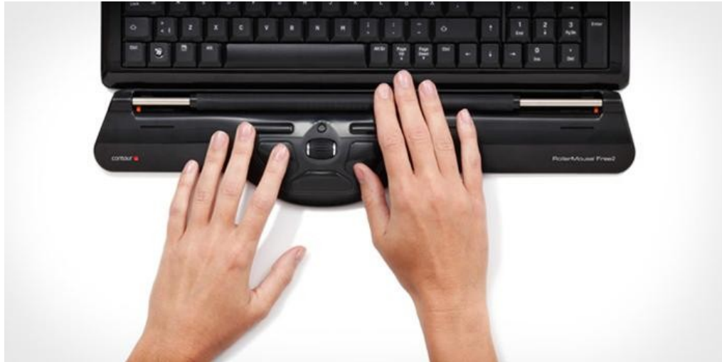
Figure 1. Rollerbar system for mouse control in front of a standard keyboard
