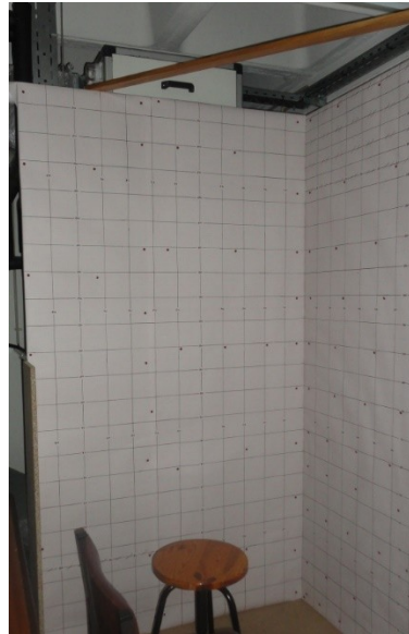
Figure 1. Stationary anthropometer with 1200 × 1500 × 2100 (depth, width, height), in mm
