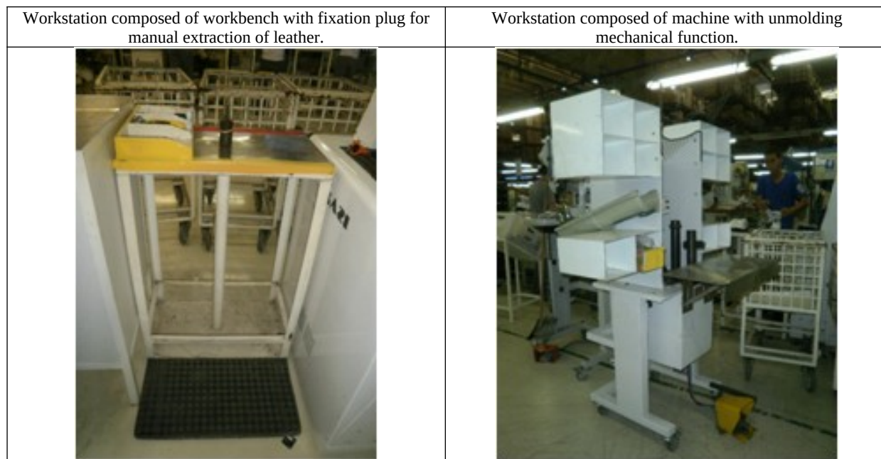
Figure 2: Workstations, constituted by benches with pin and machine, used for unmold shoe (own elaboration, 2013)
