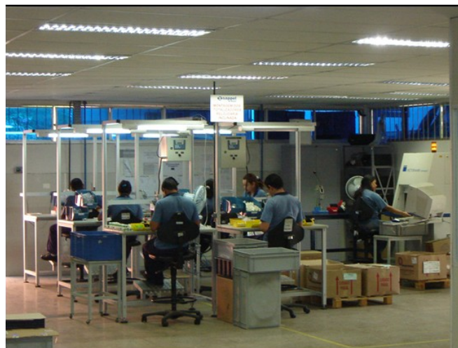
Figure 2: Mounting via layout "in cell" (collection of the author).
