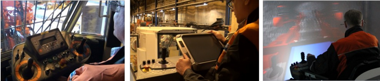
Figure 2. Observation of different cab models (real old cab, physical mock-up and digital mock-up)
