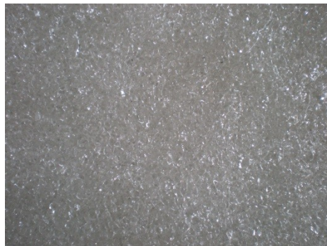
Photo 1 - Crystal piece with a partial melting which gives it the texture according to the dimension of the particle size of the broken glass. Source: Author
