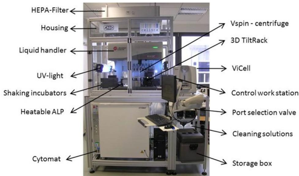
Figure 1. automated cell workstation (Lehmann R., Vetter L., Person L., Thurow K. 2013)
