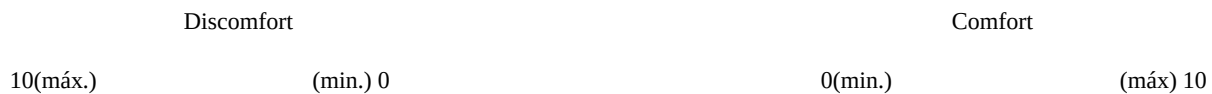
Figure 2. Separated scales for comfort and discomfort. (based on Kleeman, 1981; Kamijo, Tsujimara, Obara, & Katsumatu, 1982; Zhang, Helander, & Drudy, 1996; Helander & Zhang, 1997)
