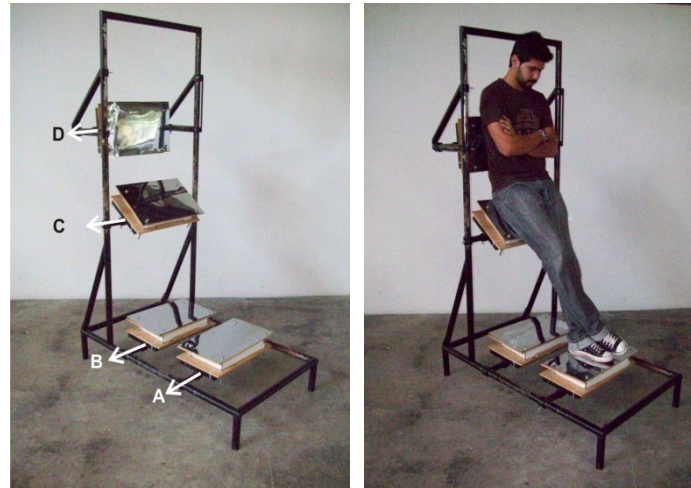
Figure 2. Dinagoniometer (DGM): A prototype designed to measure forces and angles on each axis where the points of support will be located: A and B, for feet; C, for hips; D, for shoulder, arm and back. The axes have up to three translational degrees of freedom and a one rotational degree of freedom. On the right photo, the model adopts position 4 on steel surface, by using points of support A and C.
