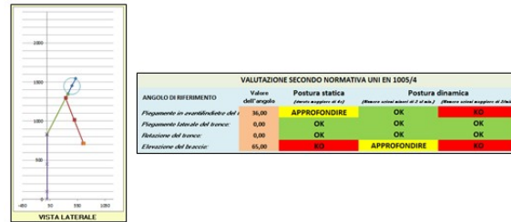
Figure 4: Sticky 2D representation of a standard virtual mannequin and its postural evaluation according to EN 1005/4 standard.
