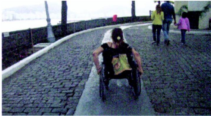
Figure 6: free track built on the original floor. Source: Cambiaghi (2007).
