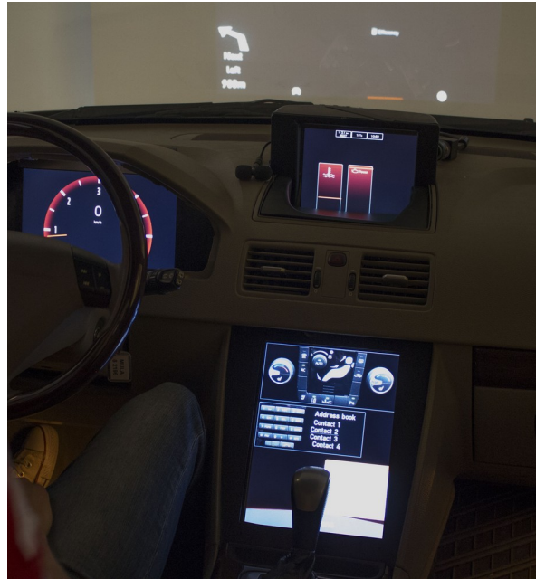
Figure 1. The user interface prototype inside the driving simulator
