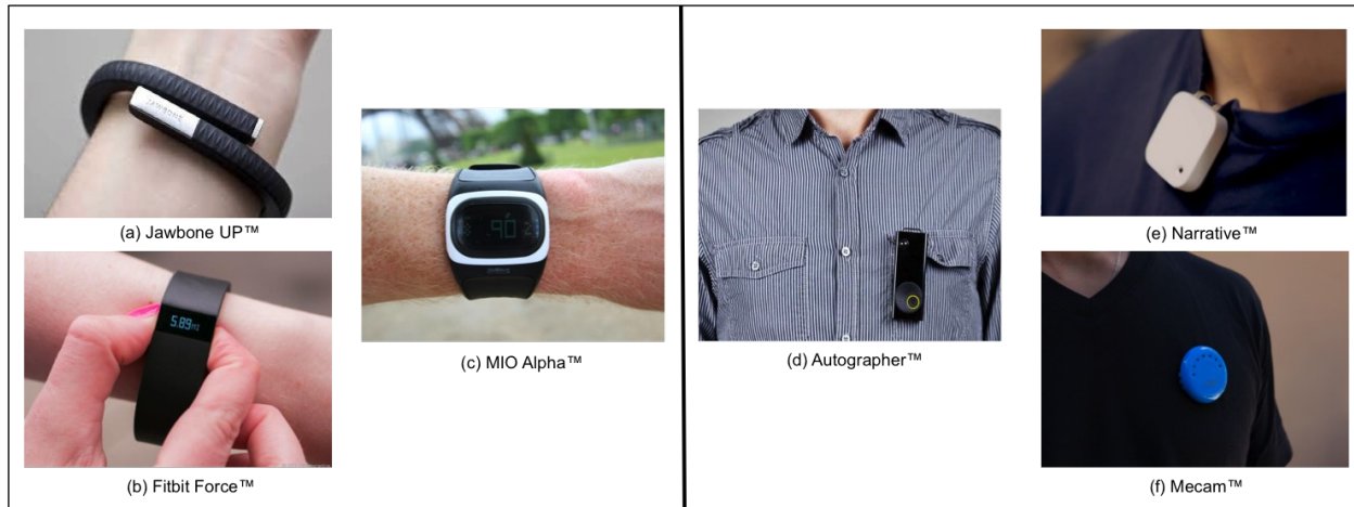
Figure 1. Wearable device as an activity tracker (Left: (a), (b), (c)) and a memory extender (Right: (d), (e), (f))
