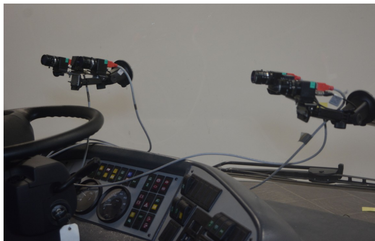
Fig. 2. Deployment of FaceLab cameras in the driver cabin during testing
