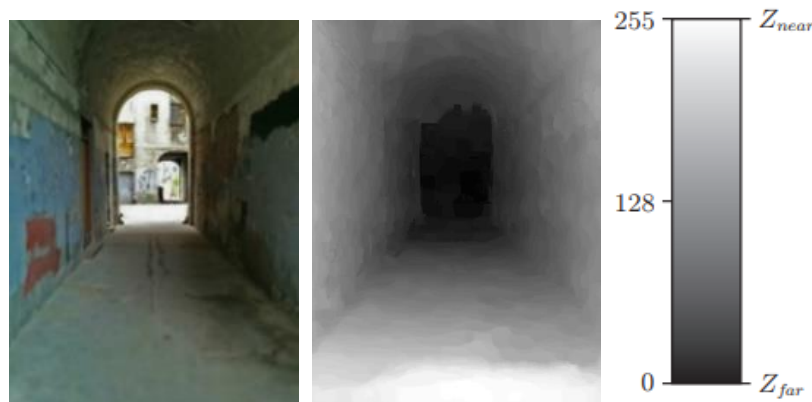
Figure 1: 2D color image (left) and 8-bit depth image (right)
