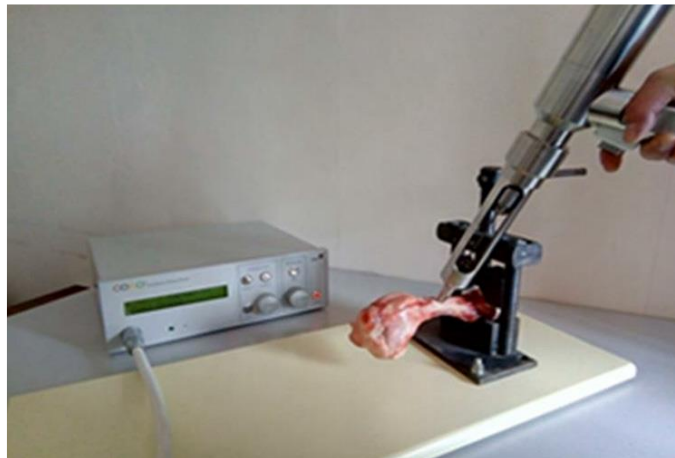
Figure 1. Setup of bone drilling execution.
