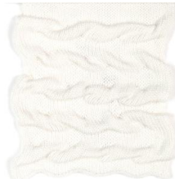
Fig. 6. Single jersey with manual manipulations that create 3D effects depending on frequency and position. Done by taking stitches already knitted back into work following a precise pattern.
