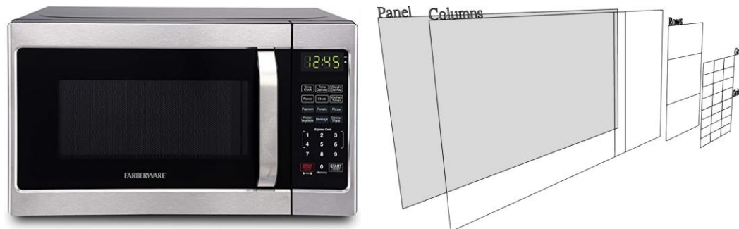
Figure 3. The UI of a microwave oven (left) and the digital representation of its layout using the proposed PUIDL (right), shown as a 3D rendering. The layout consists of a panel structured into three columns that contain the door (left), the handle (middle), and a panel (right). The latter column contains three rows: the first one contains the LED display, the second row contains a grid with push buttons for the pre-defined cooking options, and the third one contains a grid with push buttons for the numbers and the start and stop buttons.
